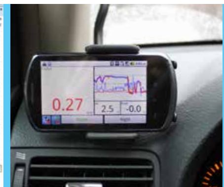
Mobile phone user interface in the vehicle. The system includes a braking friction meter application on the mobile phone.
