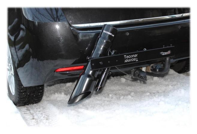
Road Condition Monitor RCM411 has been designed to be a quality control and optimization tool for winter maintenance. RCM411 is also suitable for runway condition reporting. The sensor can be installed onto a moving vehicle to follow surface conditions and friction in real time. RCM411 detects all typical surface states like:
