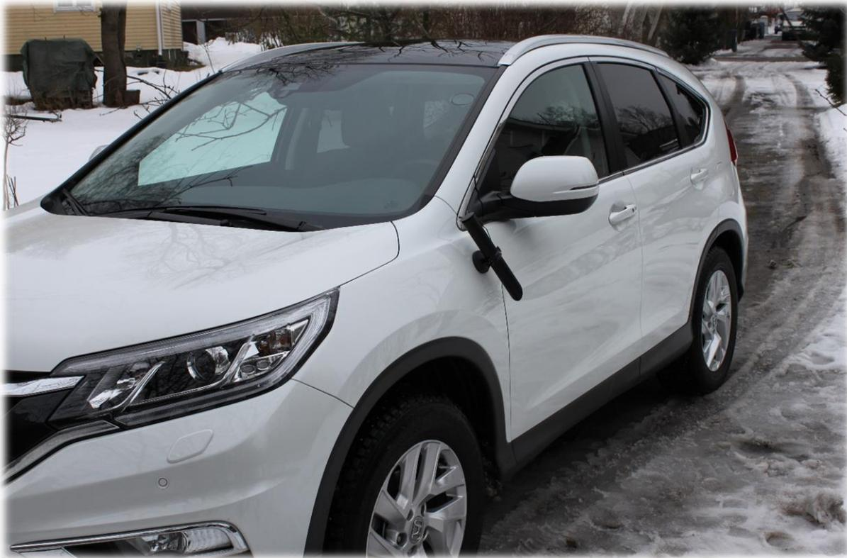
Road Surface Temperature Sensor RTS411SA is a stand-alone surface temperature sensor of Road Condition Monitor RCM411.
