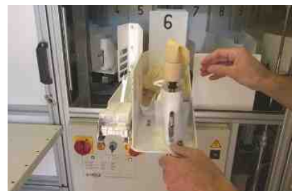
An attendant only needs to reload the daisywheel with radiosondes and balloons every 12 days.
