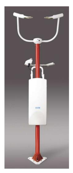
The Vaisala Present Weather Sensor FS11P is intended for demanding weather applications such as runway visual range (RVR), aeronautical and synoptical visibility and present weather observation. The FS11P is a combined RVR, visibility and present weather sensor. It delivers valuable multi-parameter measurement, all in one. It transmits data on visibility up to 75km, present weather covering obscuration, precipitation type and intensity, and optionally background luminance.
