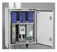
8 digital outputs and 8 digital inputs for sensors, power optimizing and unmanned control functions based on user-defined requirements.
