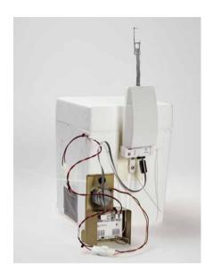
pump base. The heating is powered by an additional battery with a voltage range from 9 to 19 V. The recommended battery is a 9 V square battery that can easily be fitted onto the ozone sensor frame inside the ozone box.
